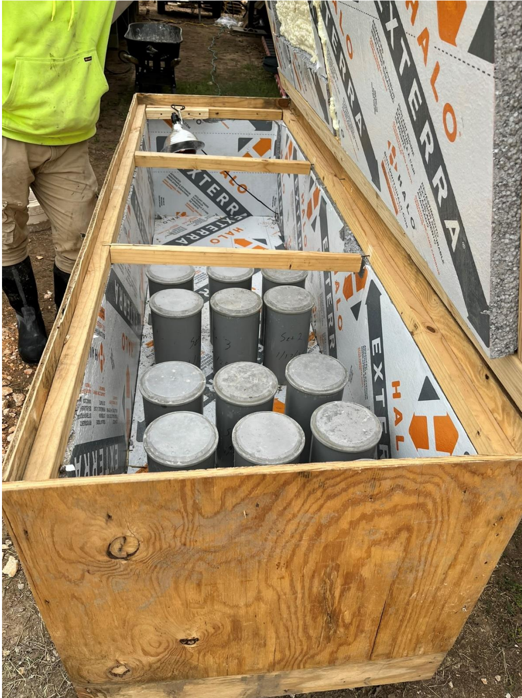
2P – Concrete Test Cylinders in controlled environment storage for cure prior to compression strength testing.
